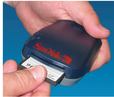
Inserting a CF card into the Holter analyser's card reader for immediate analysis
