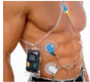
Only 3 electrodes for 3 channels of ECG
